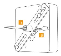
5 Make connection inside of electrical box to power wires with provided wirenuts.
