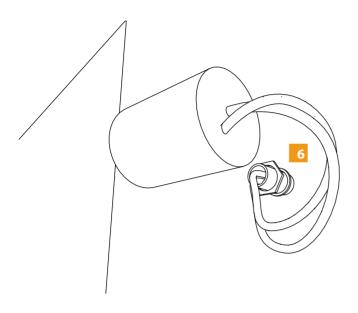
Push any excess wires through the nipple and make sure nipple is only sticking through into fixture body only as much as it needs to be to mount with hex nut.
